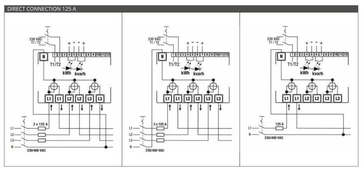
Neutral wire muste be connected to the meter
