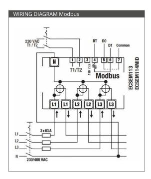
The connection of the neutral wire to the "N" terminal of the energy meter is mandatory. When the terminals RT and D0 are shorted, a termination resistor of 120  $\Omega$  is applied inside of the energy meter
