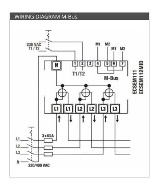
The connection of the neutral wire to the "N" terminal of the energy meter is mandatory.
