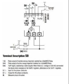
\* This fuse is recommended if neutral is not earthed. A fuse of 125 A is recommended for the line protection.
