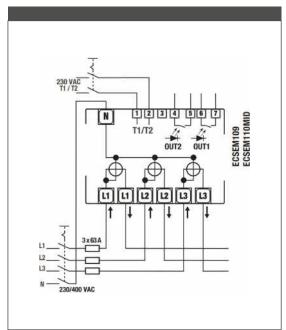
Neutral wire must be connected to the meter
