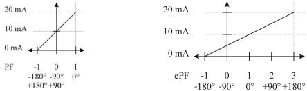
Power angle represents angle between first voltage harmonic and first current harmonic for each individual phase. Total power angle is calculated from total active and reactive power (see equation for Total power angle, chapter *Equations* on page 88). A positive sign shows inductive load, and a negative sign shows capacitive load.
