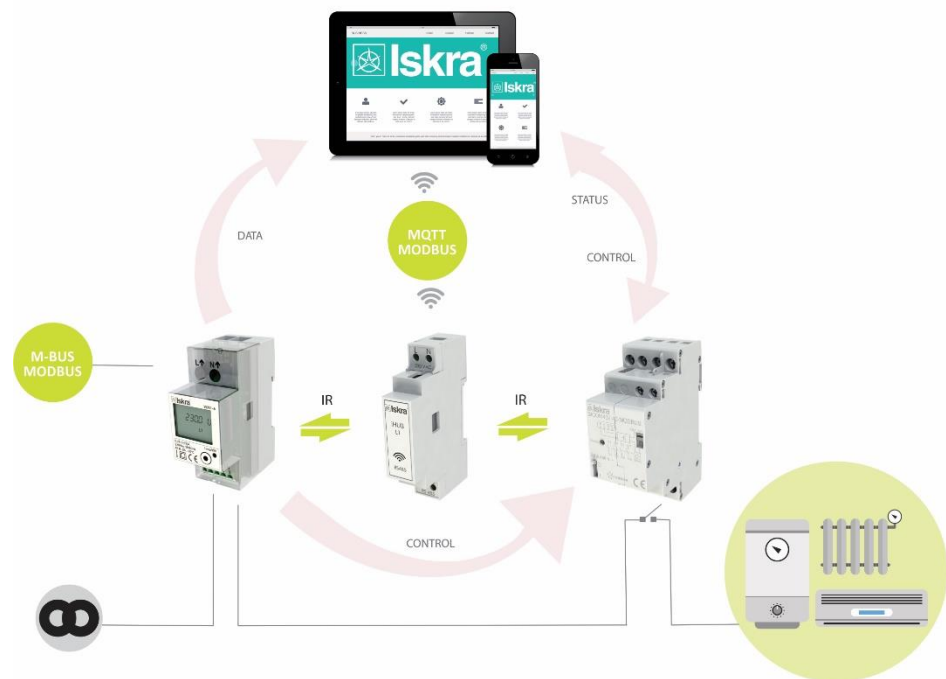
Figure 2: Connection diagram for iHUB-L1. It is connected to an energy meter (on the left side of the iHUB-L1) and to latching switch (on the right side of the iHUB-L1) by IR communication. It is possible to read and control data with the computer or mobile phone.
