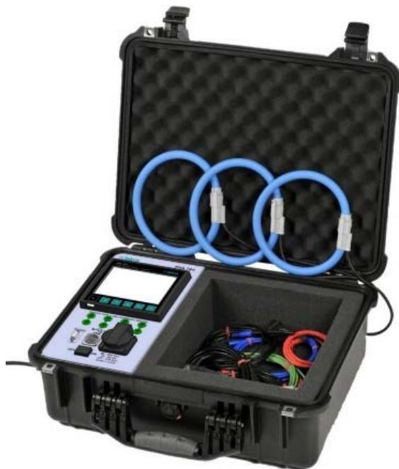
The PNA 784 network analyzer is used for analysis of electric voltage quality in compliance with the SIST EN 50160 standard. Records are stored in the internal memory. Moreover, more than 170,000 deviations of the measured quantities from the standard values are stored, which enables finding of eventual reasons for the problems on network. Optional limits and required quality in a monitored period can be defined for each monitored characteristic.
